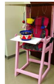
Figure 7: Assembled prototype consisting of the wooden base, adjustable table, car seat, game on the table, and hanging apparatus
