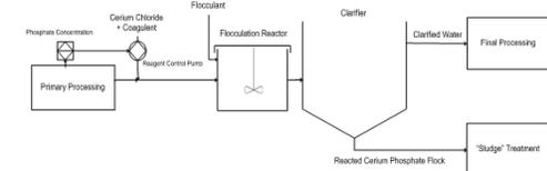
Figure 7: Displays the designed process flow diagram of a cerium-salt based water treatment plan. This process consists of evaluating the phosphate concentration of primarily processed wastewater, using a pump to deliver the reagent, adding and agitating the flocculent and then separating the clean water from the flock in a clarifier. Additives will be dependent on water source.
