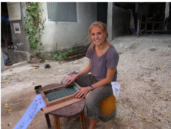
Screen Printing at moussa's workshop, made the screen out of shoe tacks and silk fabric, printed on scrap fabric.
