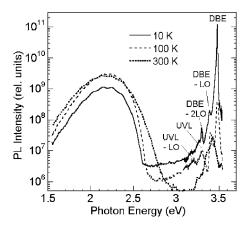
FIG. 1. PL spectrum from a GaN layer at different temperatures. The QE of different PL bands:  $\eta_{\text{exciton}}=8\%$  at 10 K;  $\eta_{\text{YL}}=2\%$  at 10 K and 4% at 100–300 K;  $\eta_{\text{UVL}}=0.01\%$  at 100 K.
