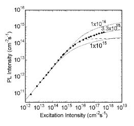
FIG. 2. Dependence of the YL intensity on excitation intensity at 300 K. Points—experimental data. Solid lines—calculated by using Eq. (6) with the following parameters:  $\alpha = 10^5$  cm<sup>-1</sup>,  $\tau = 0.4$  ms,  $\eta_{YL}^{exc} = 0.04$ ,  $N_{YL} = 1 \times 10^{15}$ ,  $3.3 \times 10^{15}$  and  $10 \times 10^{16}$  cm<sup>-3</sup>.
