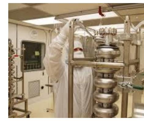
To achieve this, a set of coils are wrapped around the testing cavities. When current is driven through the coils, a magnetic field is created that opposes the magnetic field from the building, thus neutralizing it. To optimize this method, an accurate reading of the uncompensated magnetic field must be taken. This data is used to create a field that will exactly negate the building's magnetic field.
