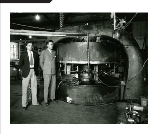
The building that now holds the vertical testing area at Jefferson Laboratory was once occupied by the Space Radiation **Effects Laboratory in the 1960's. This** laboratory had a cyclotron, which is a type of particle accelerator. As a result of this, the rebar within this particular building is now slightly magnetized.
