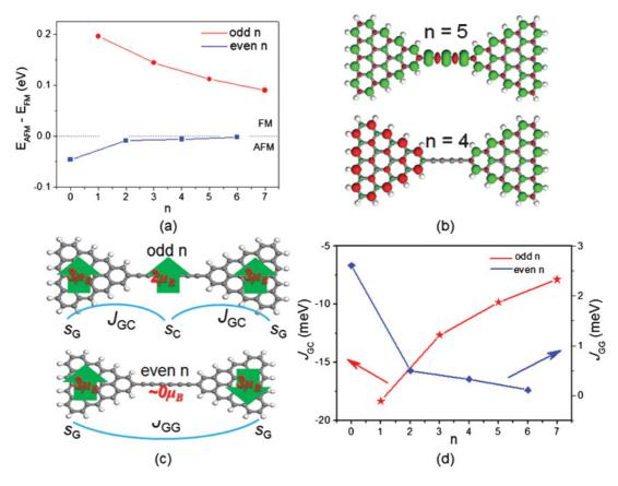
FIG. 2. (Color online) (a) Exchange energy  $(E_{AFM} - E_{FM})$  as a function of C chain index *n*. (b) Spin density of GNF<sub>5</sub>-C<sub>5</sub>-GNF<sub>5</sub> in FM and GNF<sub>5</sub>-C<sub>4</sub>-GNF<sub>5</sub> in AFM states. (c) Sketch of Ising model describing magnetic behavior with exchange parameters for odd and even *n*. (d) Simulated variation of  $J_{GC}$  and  $J_{GG}$  parameters with index *n*.
