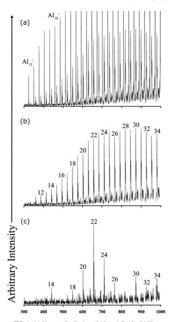
FIG. 1. (a) Nascent distribution of  $Al_n^-$  and  $CuAl_n^-$ . (b) Nascent  $CuAl_n^-$  distribution (c) Oxygen-etched  $CuAl_n^-$  distribution (1.25% partial pressure of oxygen). Peaks corresponding to pure aluminum clusters were superficially removed from (b) and (c) to discriminate  $CuAl_n^-$ .
