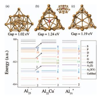
FIG. 4. (Color) Geometry and HOMO-LUMO Gaps of (a)  $Al_{23}^-$ , (b)  $CuAl_{22}^-$ , and (c)  $Al_{23}^+$ . Below, the electronic structure of (a), (b), and (c) with labeled shells.  $A_1(XY)$  and  $A_1(Z)$  indicate hybridized levels with extra nodes along the XY and Z planes.
