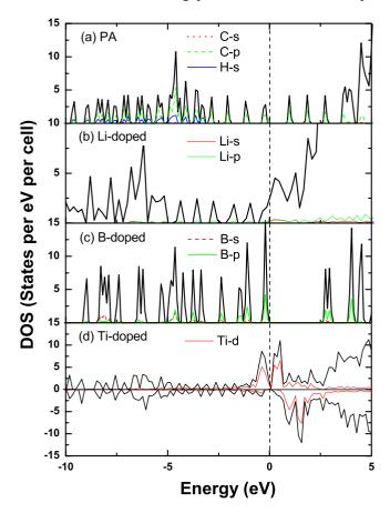
FIG. 2. (Color online) Calculated density of states for intrinsic, Li-doped, B-doped, and Ti-doped cis-PAs; the black solid lines represent the total density of states; Fermi level is set at zero.
