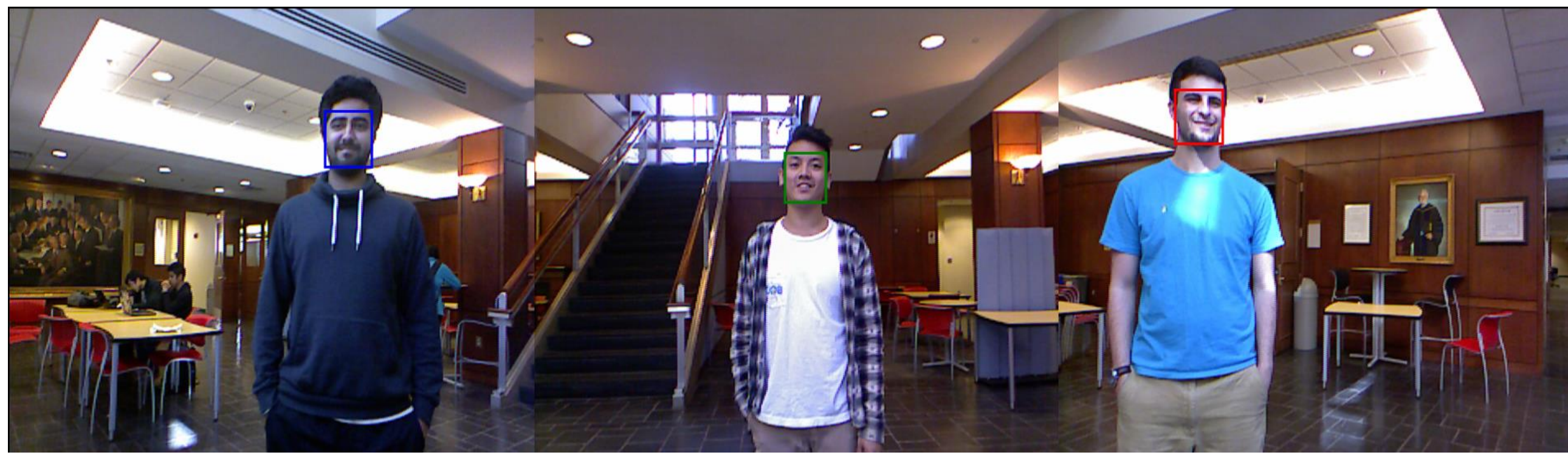
Figure 4 – Demonstrates Face Tracking capability across integrated sensors simultaneously. Notice each face is a different tracking color representing person identification.
