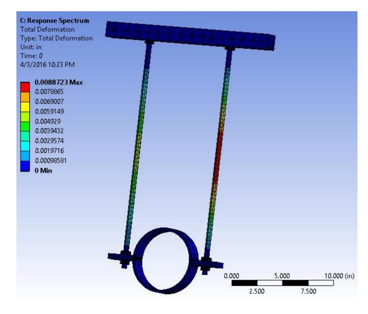
Below shows a maximum total stress of 6014 psi create by the load and velocities, which is well below the tensile and compressive yield strength
