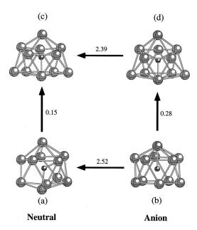
FIG. 4. Isomeric structures of neutral and anionic Al<sub>II</sub>C clusters showing the energies required to go from one structure to the other. The lower row gives the ground states and the upper row presents the lowest lying isomers.
