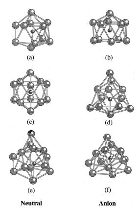
FIG. 3. Ground state geometries of neutral and anionic  $Al_nC(n = 11, 12, 13)$  clusters obtained from 6-311G\*\* basis.
