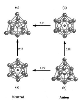
FIG. 2. Isomeric structures of neutral and anionic  $Al_{12}C$  clusters showing the energies required to go from one structure to the other. The lower row presents the ground states while the upper row shows the lowest lying isomers. The results correspond to the all-electron calculations using the  $6-311G^{**}$  basis.
