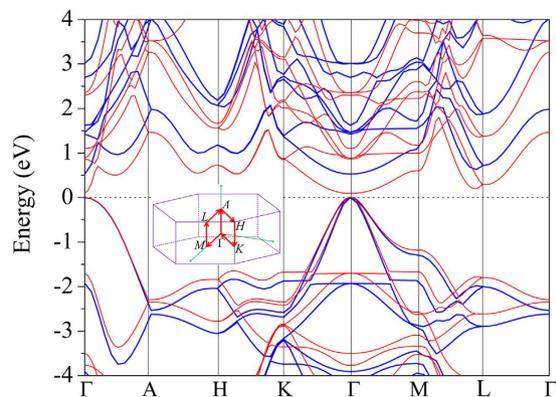
**Figure 3. Electronic Properties.** Calculated band structure of h-Si<sub>6</sub> (red lines: GGA/PBE; blue lines: HSE06) with the Fermi level set to zero. The high symmetry *k*-point path in the Brillouin zone is shown in the inset.
