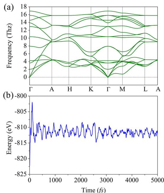
**Figure 2. Structural stability of h-Si<sub>6</sub>.** (a) Phonon dispersions and (b) energy fluctuation of h-Si<sub>6</sub> with respect to time in MD simulations at 500 K.
