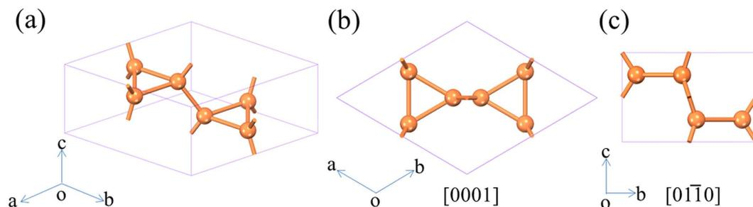
**Figure 1. Optimized crystal structure of h-Si<sub>6</sub>.** (a) Perspective view, (b) view from the [0001] direction, and (c) view from the [0110] direction.
