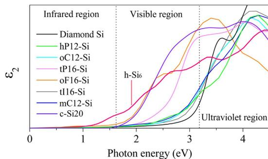
**Figure 4. Optical properties.** Imaginary part of dielectric function for h-Si<sub>6</sub>, diamond silicon, and other metastable silicon allotropes calculated at the HSE06 level.
