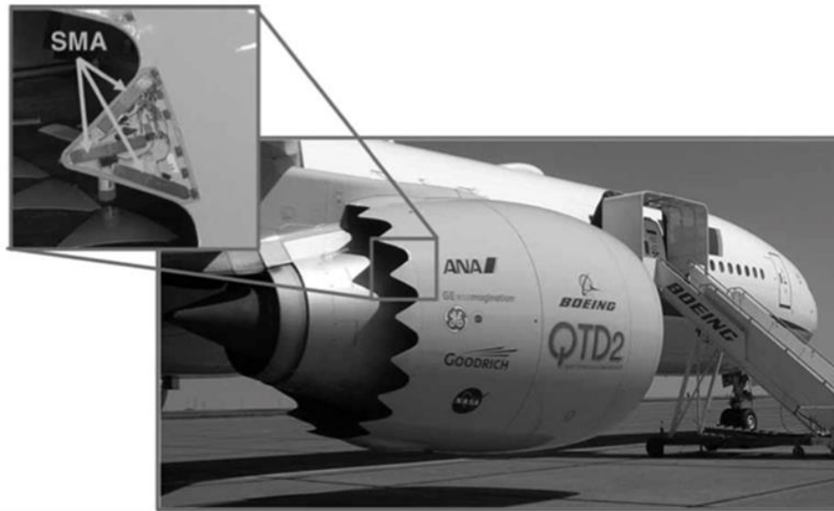
Figure 1.11: SMA beams as chevrons [8]
