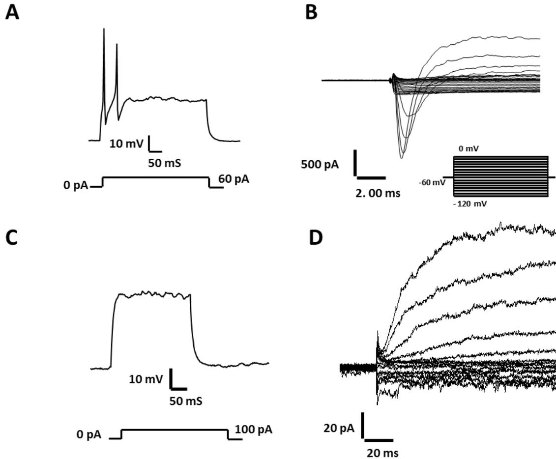
**Figure 14: Electrophysiology of enteric neurons:** A) Current clamp recording from a neuron showing an action potential with a current stimulus of 60 pA C) Current clamp recording from a glial cell showing no action potential with a current stimulus of 100 pA. B) Whole-Cell voltage clamp recordings from neurons showing inward sodium current induced upon giving a series of voltage steps from -120 mV to 0 mV. D) Whole-cell voltage clamp recording from a glial cell without any inward currents.
