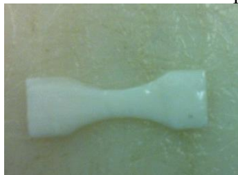
Figure 4: Preparation of specimens for uniaxial tensile testing - Preparation of samples into “dog bone” specimens measuring 2.75mm wide at their narrowest point with a length of 7.5mm
