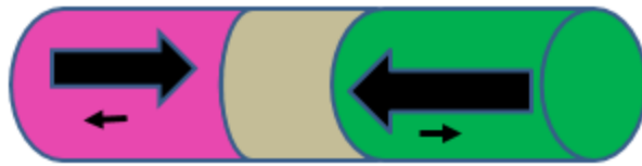
Figure 2-12: Current conduction in a nanowire spin valve
