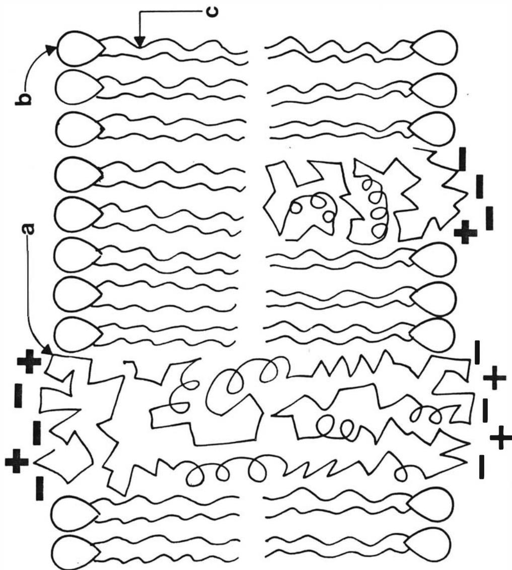
Figure 2. Model of the electrode-solution double layer (9).
