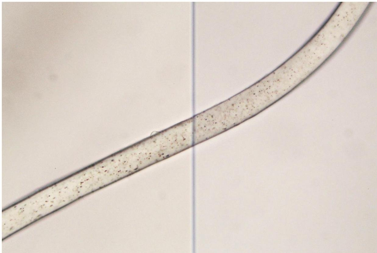
**Figure 24.** Two Physically & Optically Similar Fiber Samples Side-by-Side on the Comparison PLM, 400x Magnification.
