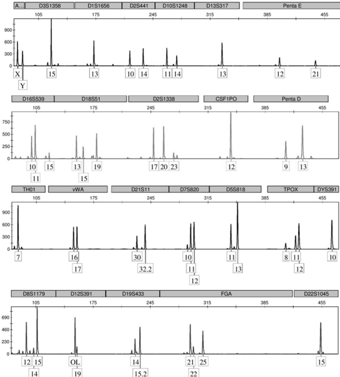
**Figure 7** - Representative electropherogram for 50 cells isolated from a reconstituted swab semen/vaginal fluid mixture demonstrating full profile development with no degradation. Some drop-in is observed.
