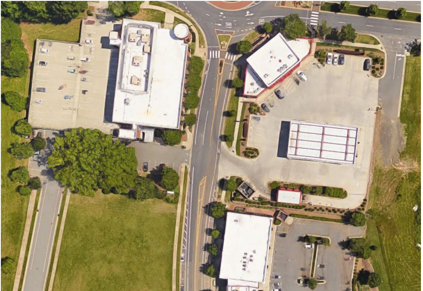
Figure 22. Two stores along a major crossroads at a roundabout in Davidson, North Carolina. The service station on the right has a partial entrance road that could be extended later when the next parcel is developed (Source: Google Maps, 2019.)
