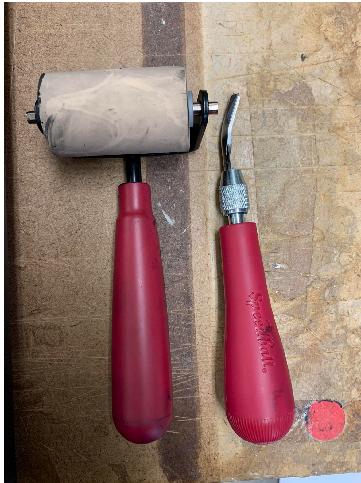
TOOLS USED TO CARVE AND ROLL INK ONTO THE STAMP
