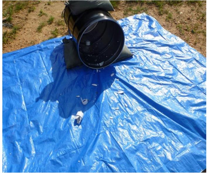
**Figure 2:** Before and after the water column was used to disrupt the PVC mock IED. The pieces inside the barrel and on the tarp were collected separately.
