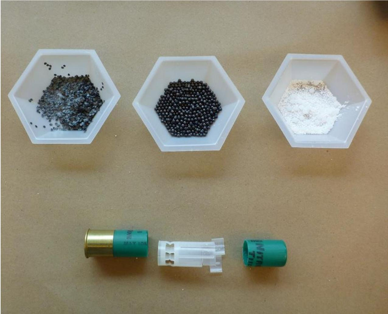
**Figure 27:** Disassembled Remington NitroTurkey shotgun shell used in the PAN disrupter that propels birdshot down the barrel.
