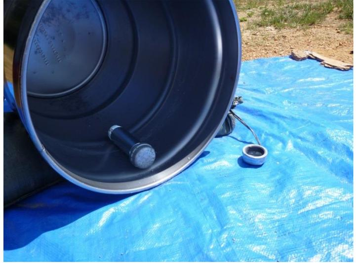
**Figure 3:** Before and after the birdshot was used to disrupt the steel mock IED. The pieces inside the barrel and on the tarp were collected separately.
