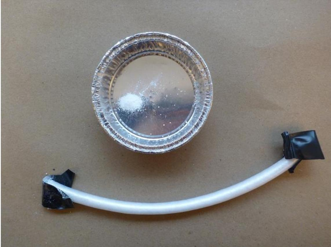
**Figure 40:** Detonation cord utilized in the Mineral Bottle. A small amount of the high explosive powder used in the cord was collected into the metal tray. The ends are taped to prevent the cord from losing powder.
