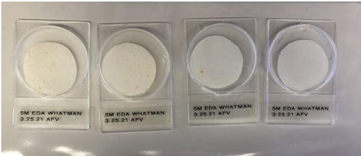
Figure A17. 5M EDA filters with sprayed TNT at different distances.
