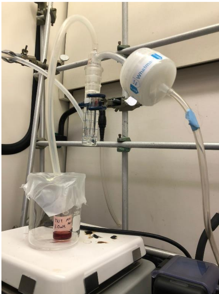
Figure A16. Impinger method set-up.
