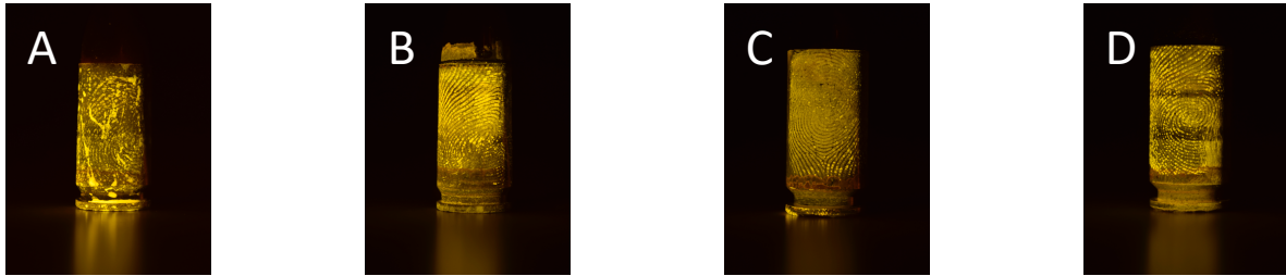
Figure 2. Photos of the positive controls on a: a) brass case 9mm Luger cartridge; b) nickel case 9mm Luger cartridge; c) brass case 40 S&W cartridge; d) nickel case 40 S&W cartridge. Taken with a Nikon DSLR camera model D3300 using a Nikon AF-P DX NIKKOR 18-55mm lens and a 52mm PROMASTER orange (YA2) filter.
