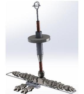
Figure 5: Actively Cooled Grid Design
