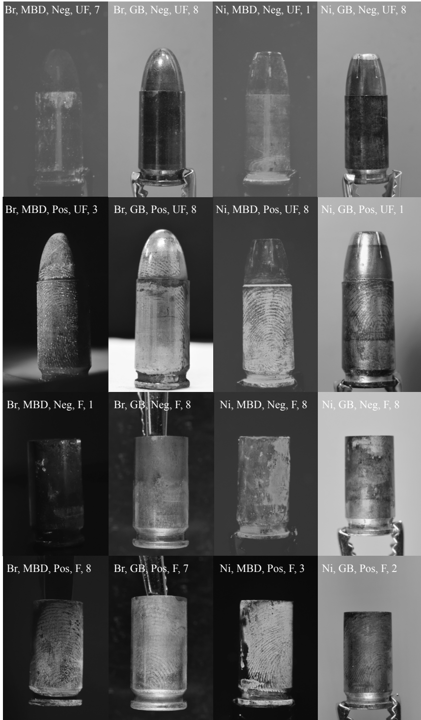
Figure 1. Positive and Negative Control Results. Br: brass, Ni: nickel-plated, GB: bun glue processed, MBD: MBD dye stain processed, Pos: positive control, Neg: negative control, UF: unfired, F: fired, #: sample number of cartridge case shown.
