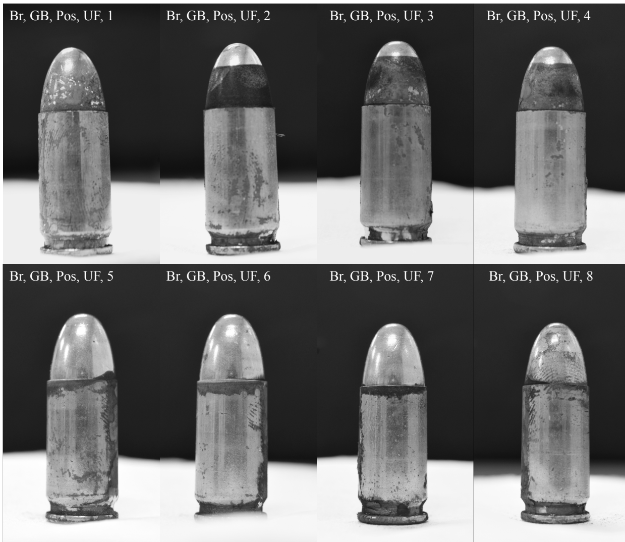
Figure 4. Failure of Gun Bluing Method on Unfired Brass Cartridge Cases. Br: brass, GB: bun glue processed, Pos: positive control, UF: unfired, #: sample number of cartridge case shown.
