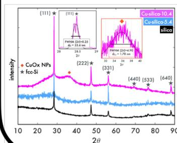
Left: XRD patterns of Cu-silica-10.4, Cu-silica-5.4, and silica generated from ablating a silicon wafer immersed in water. Inset shows FWHM fitting of peaks, with the particle diameter determined using the Scherrer equation.<sup>3</sup>
