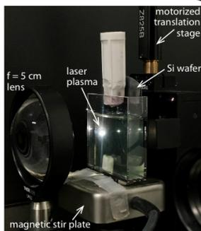
Ablated silicon wafer immersed in aqueous Cu(NO<sub>3</sub>)<sub>2</sub> solutions (2 mM) with:
