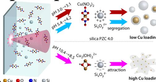
Low and medium solution pH: ablated silica clusters (oxidized silicon atoms upon interaction with water) are protonated, repel nearby Cu<sup>2+</sup> ions, resulting in low wt.% loading of Cu, and Cu-core/silica-shell morphology
