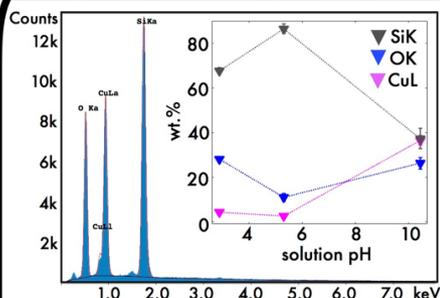
Left: Representative SEM-EDS spectrum of Cu-silica-10.4 sample. Inset shows wt.% Si, O, and Cu quantified in samples fabricated from different pH solutions
