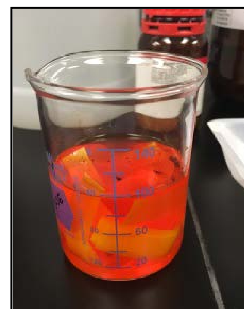
Creation of test strips in bromocresol purple bath
