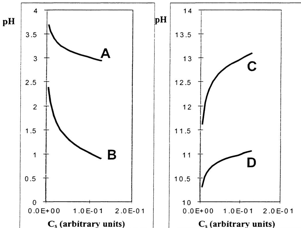
**Figure 1.** Plots of pH as a function of solute concentration. A: Vinegar; B: Hydrochloric Acid; C: Sodium Hydroxide; D: Glass Cleaner (Windex®).
