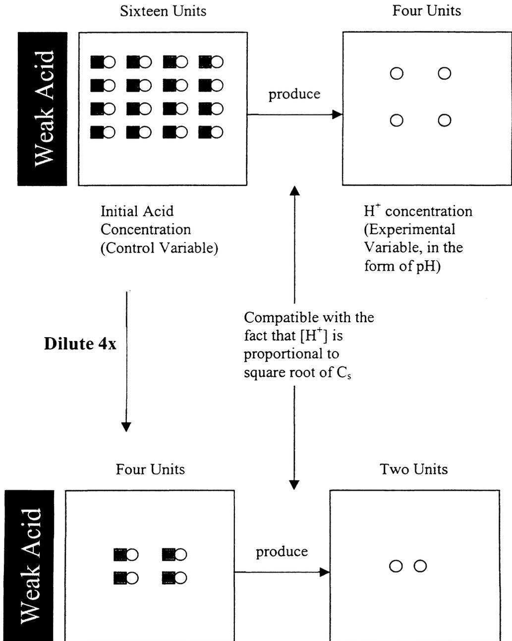
**Figure 3b.** Microscopic view of the dilution of a weak acid and its effect on  $H^+$  concentration.
