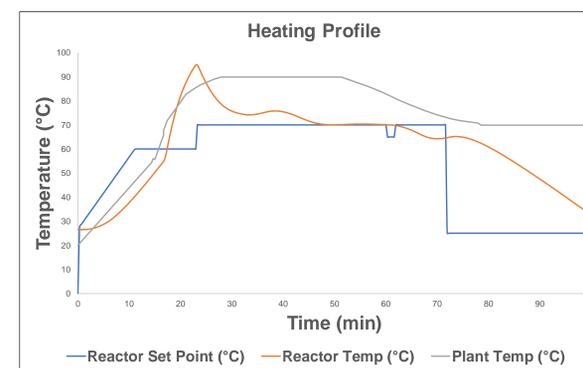
Figure 3. Heating profile for polyether in lab-scale reactor
