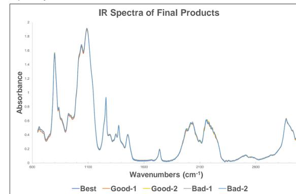
Figure 2. IR spectra for products of various quality. All products returned the same spectra and overlap on the graph, showing that IR would **not** be a viable test to differentiate products of varying quality.
