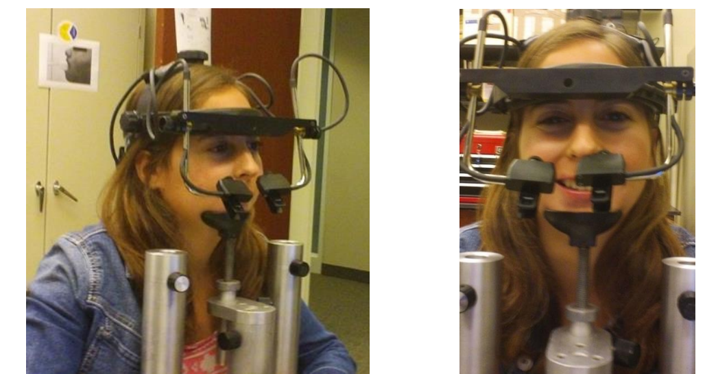
Figure 5. The eye tracker bathes the viewer's eyes with infrared light. The reflection of the light off the pupil is captured by the cameras and used to calculate the position of the eye.
