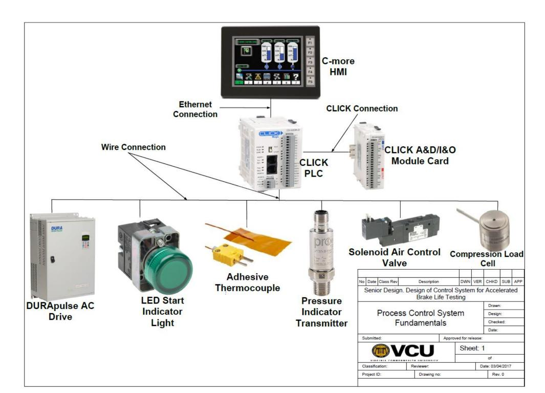
All prior electrical systems will be removed in order to update the entire structure for the new components. Click PLC (Programmable Logic Controller) C-more HMI (Human-Machine Interface) VFD (Variable Frequency Drive) Pressure Transmitter Thermal Transmitter Load Cell Transmitter **LED Start Indicator Switch**
