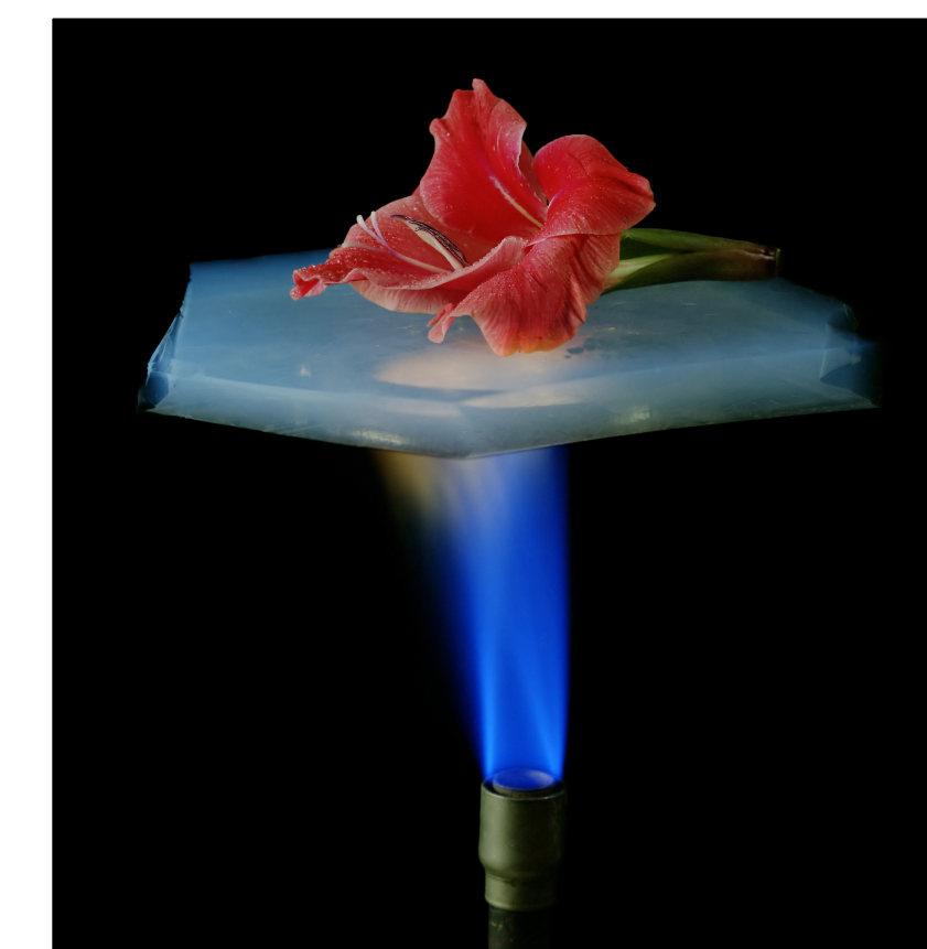
Image 3: A piece of aerogel insulation protecting a flower from a torch
