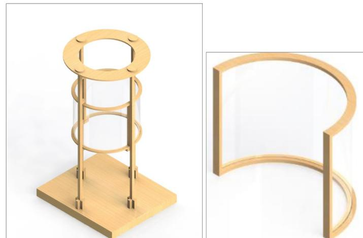
**Air Immobilization:** Air was chosen for immobilization because radiation can easily flow through air and it allows so there are no physical interferences while the radiation is being applied.
