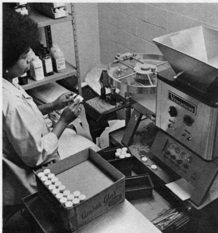
Mrs. Sylvia Johnson operates machine which automatically counts pills in selected numbers and fills pharmaceutical bottles. Each bottle is then labeled for distribution to hospital floors.
