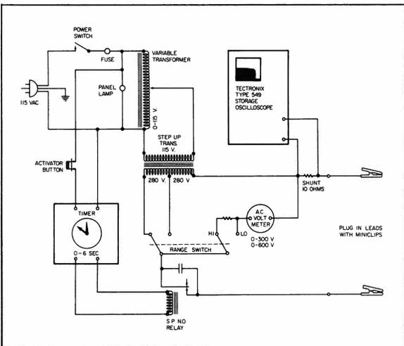
Fig. 7—Wiring diagram of experimental apparatus.
