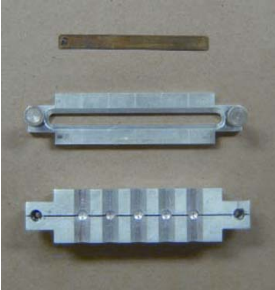
Figure 2. Custom aluminum jig for aligning castings to index for soldering. The jig consists of 2 structures that fit precisely together to hold 10 castings (5 on each side) with a gap distance produced by a leaf gauge.
