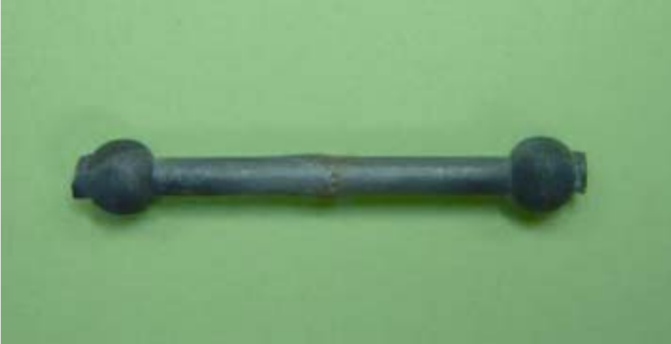
Figure 4. Typical tensile test specimen before machining.
