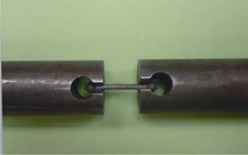
Figure 5. Tensile test specimen in holding apparatus on Instron testing machine.
