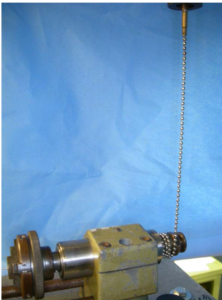
Instron Set Up. Lathe with axle attached ball and clasp chain. File handle can be seen in chuck on left. Chain attaches to 50 pound load cell superiorly.
