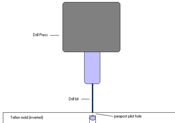
**Figure 2** Drilling Pilot Hole for Plastic Burnout Post Placement
