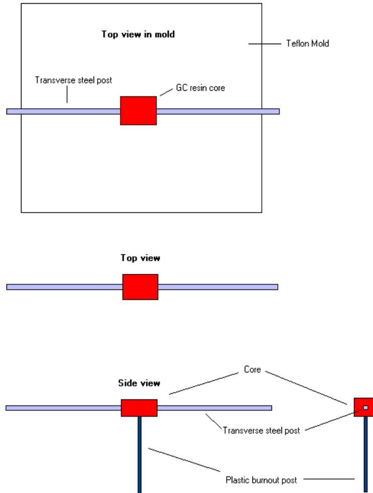
**Figure 1** Illustration of Custom Teflon Mold for Dowel-Core Fabrication
