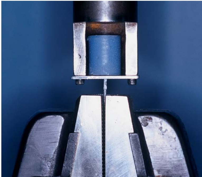
Figure 2b: Post Pulled Out of Canal
