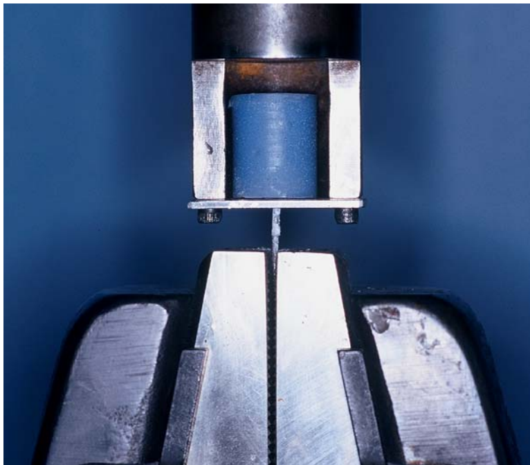
Figure 2b: Post Pulled Out of Canal
