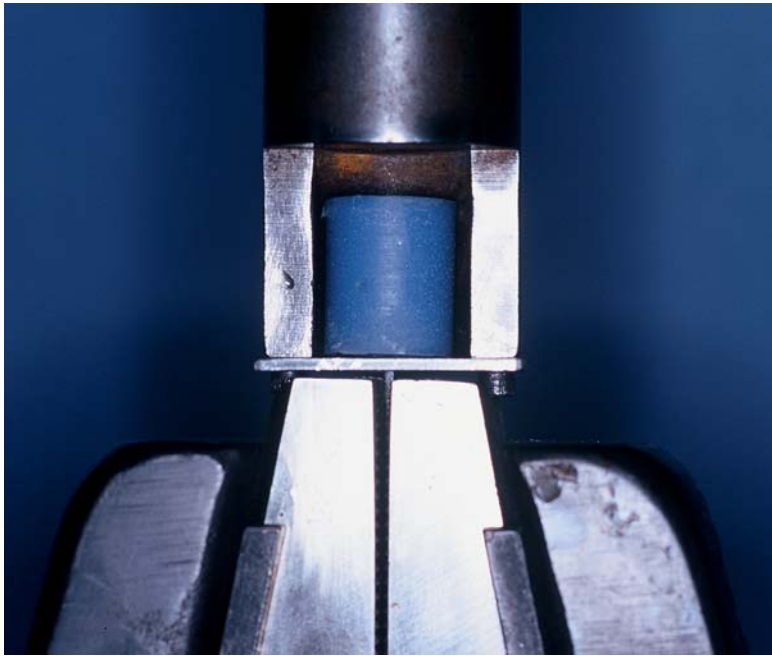
Figure 2a: Post Retention Specimen Positioned in the Instron Machine
