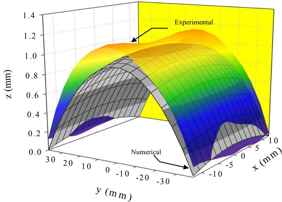
**Figure 23: Surface Topology Data for Lipca C2**
