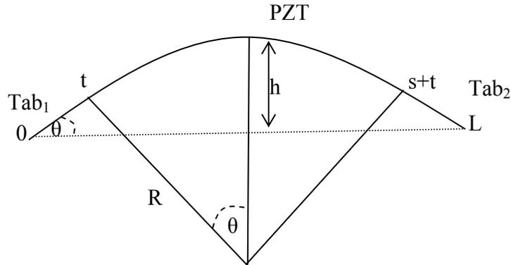
**Figure 9: Actuator geometry with flat tabs**
