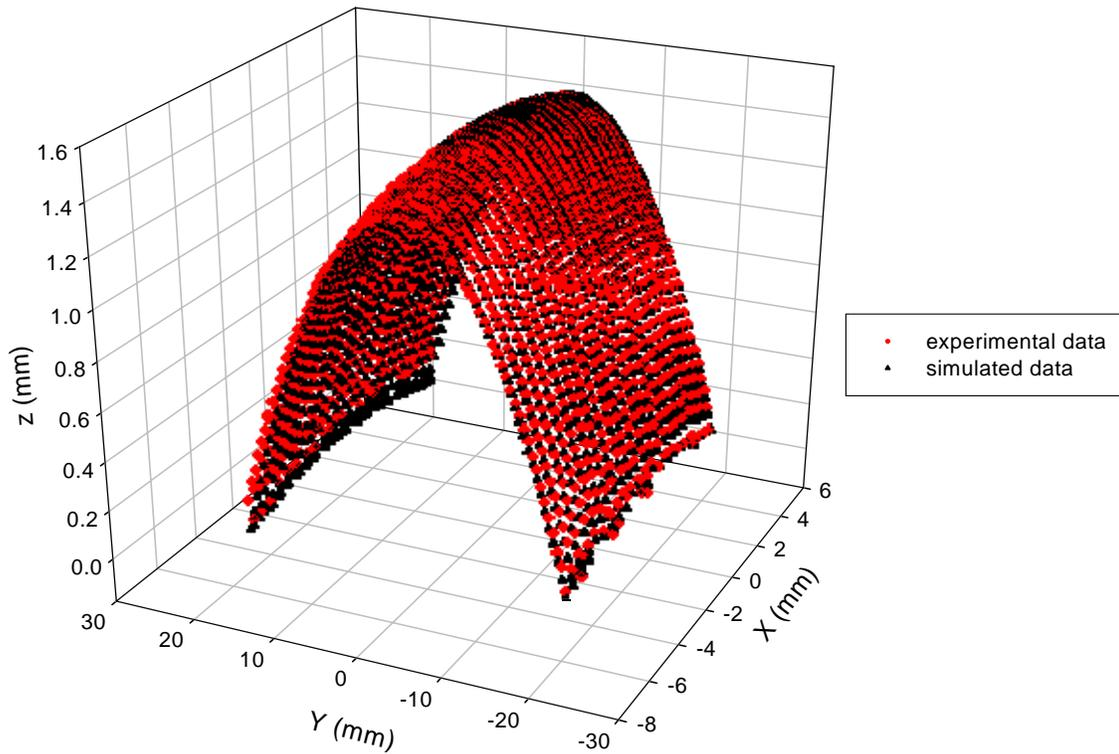
**Figure 27: Thunder<sup>®</sup> 8R Experimental and Simulated Shape**
