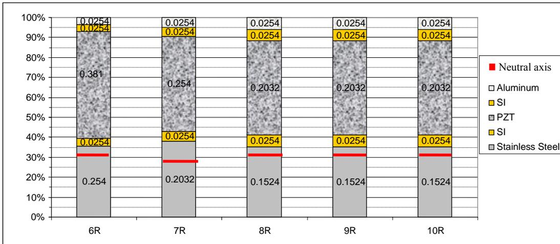
Figure 15: Neutral Axis Location for Thunder<sup>®</sup> Actuators
