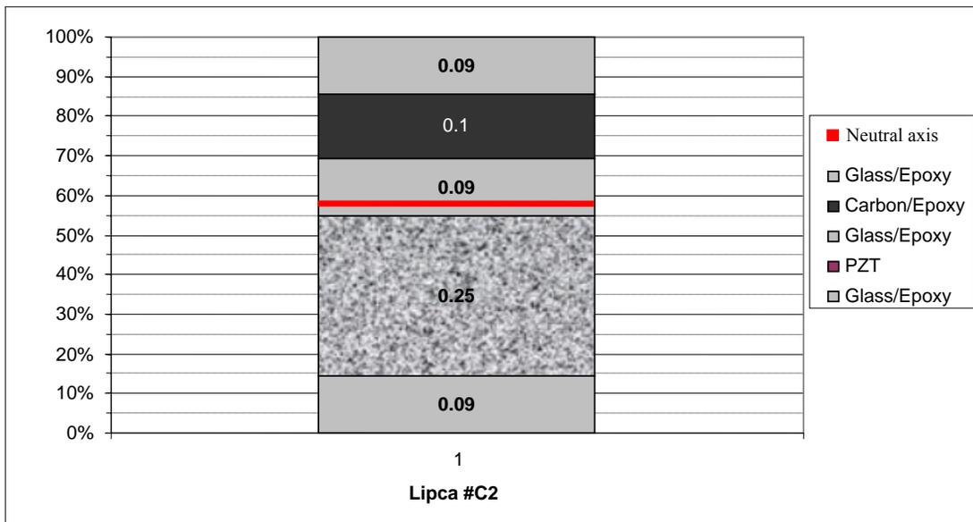
Figure 16: Neutral Axis Location for Lipca C2 Actuator
