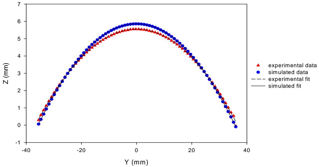
Figure 31: 2D Plot of Thunder<sup>®</sup> 7R Experimental and Simulated Shape
