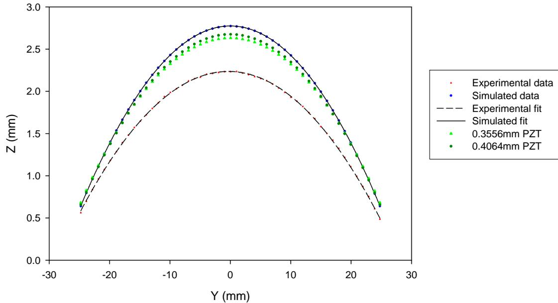
**Figure 35: Effect of PZT Tolerance on Thunder<sup>®</sup> 6R Simulation (2D)**
