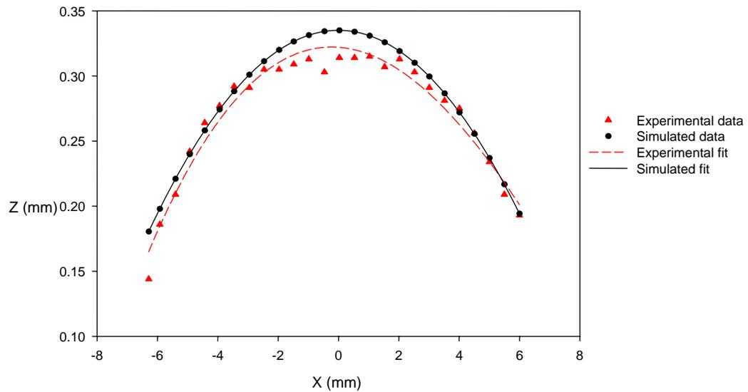
**Figure 34: 2D Plot of Thunder<sup>®</sup> 10R Experimental and Simulated Shape**
