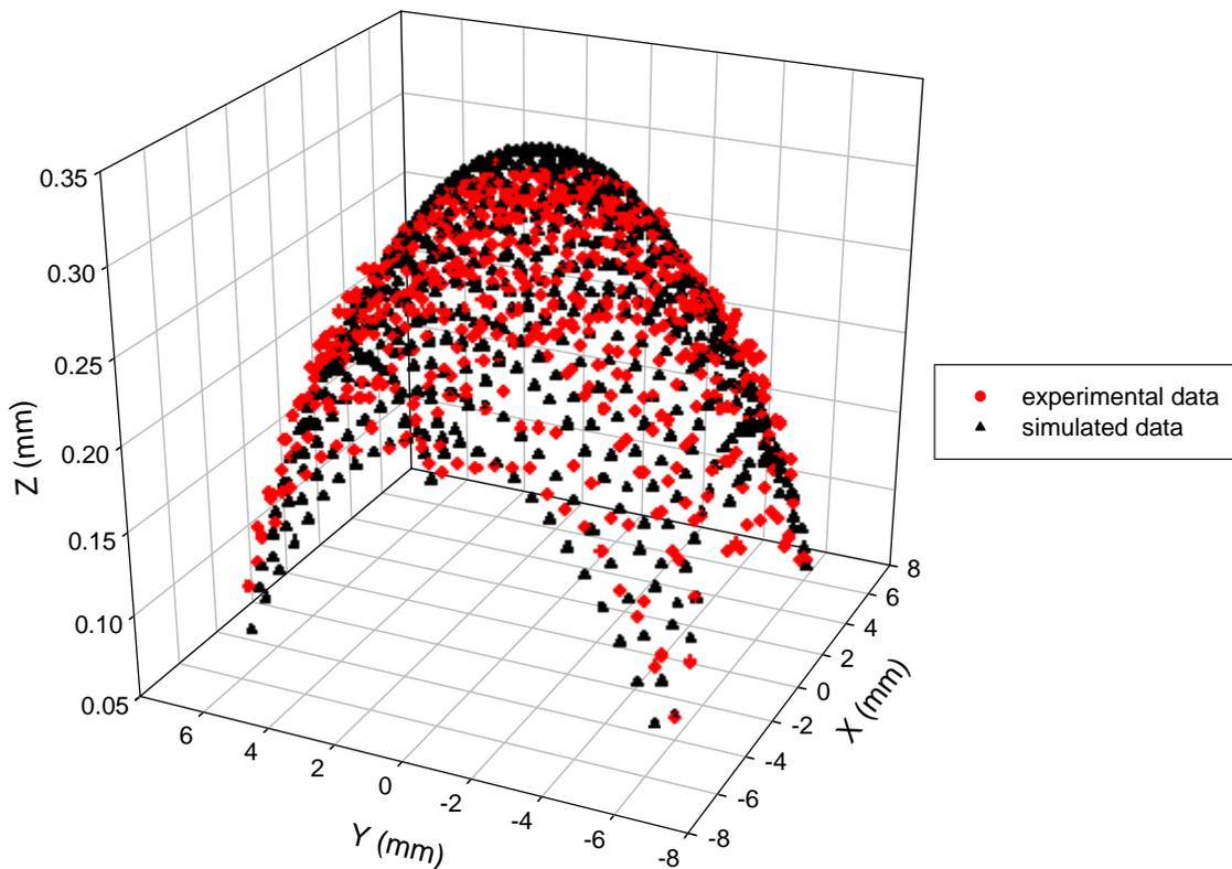
**Figure 29: Thunder<sup>®</sup> 10R Experimental and Simulated Shape**
