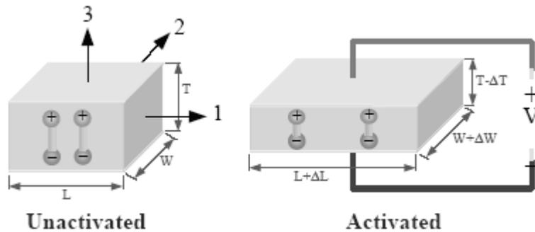
**Figure 1: A Piezoelectric Response to an Electric Field**
