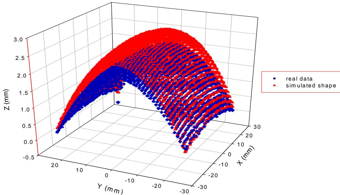
**Figure 24: Thunder<sup>®</sup> 6R Experimental and Simulated Shape**
