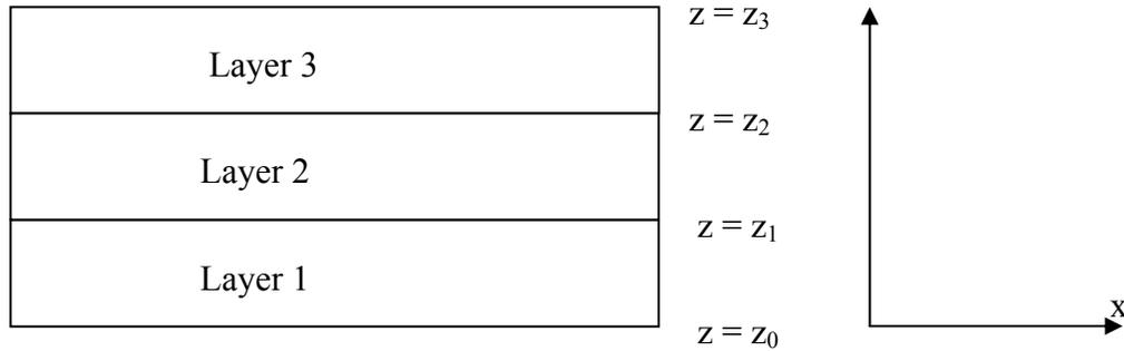
**Figure 7: Cross-Sectional Geometry of a Piezoelectric Composite**
