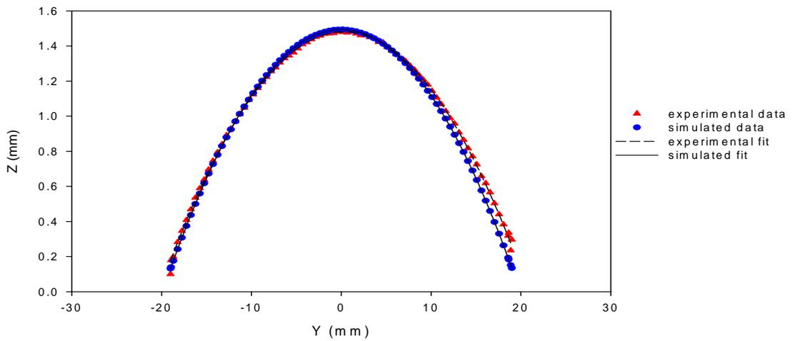
Figure 32: 2D plot of Thunder<sup>®</sup> 8R Experimental and Simulated Shape
