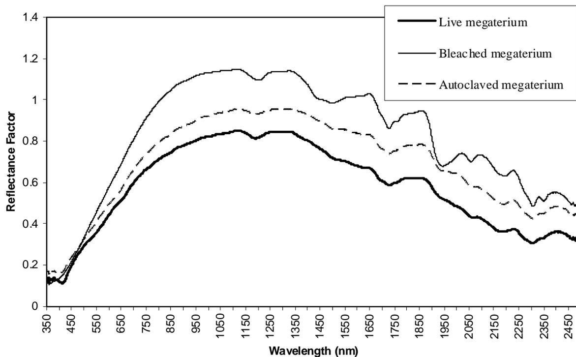
**Figure 4.** Example spectra for treated and non-treated spores of *B. megaterium*. Each sample spectrum consists of an average of five spectra, representative of the entire sample surface. Live spores exhibit deeper absorption in the area of interest (AOI) (380nm-450nm) than both autoclave-treated and bleach-treated spores.
