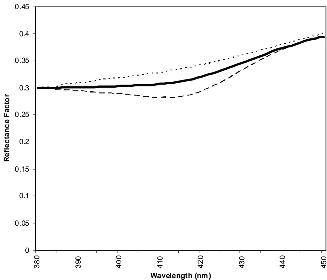
**Figure 3.** This is an example of the Grand Average Integration (GAI) method. The bold spectrum represents the “grand average” spectrum. The broken lines are examples of sample spectra. Integrals calculated for spectra below the grand average had negative values while those above had positive values.
