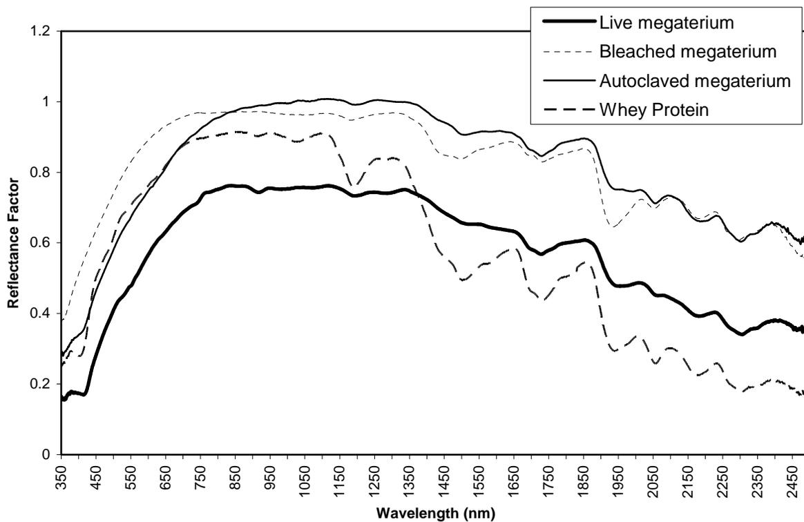
**Figure 6.** Similarities in reflectance absorptions between whey protein powder and both treated and untreated endospores. Identical absorptions are found at 410 nm, 910 nm, 1020 nm, 1510 nm, 1690 nm, 2060 nm, and throughout the short-wave infrared (SWIR).
