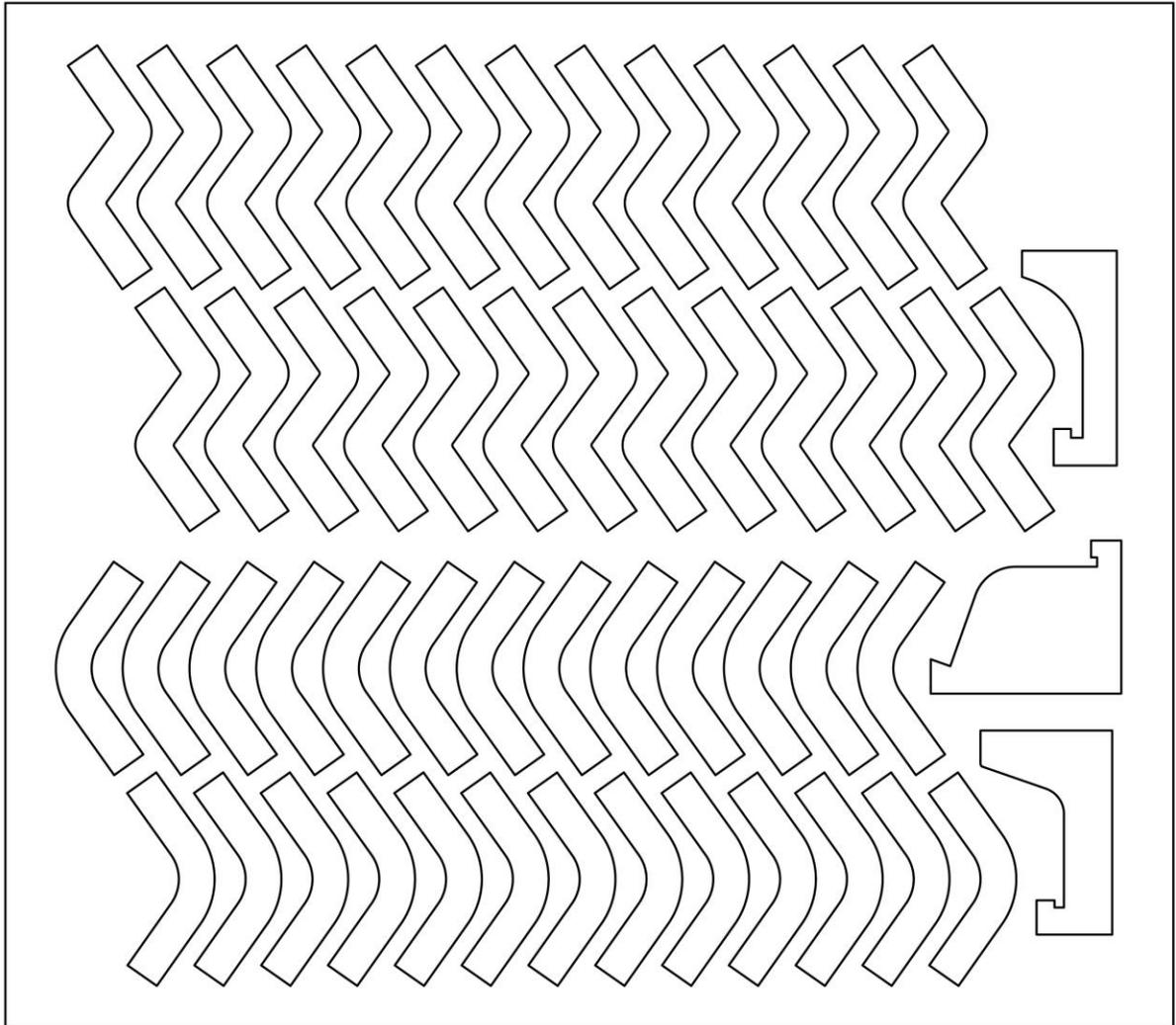
**Figure 1: Typical arrangement of parts and jigs on a sheet of half inch MDF.**
