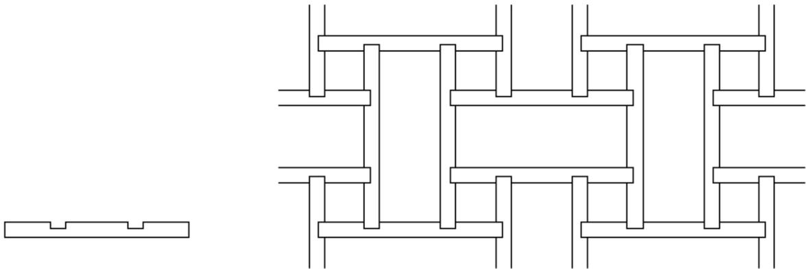
**Figure 4: Square mirrored counterchange lattice and its component part.**
