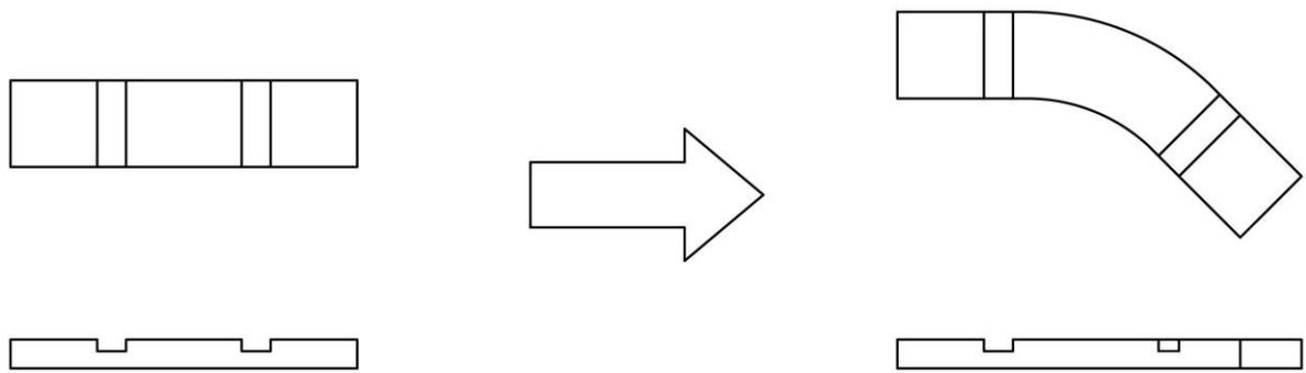
**Figure 9: Counterchange lattice part bent to facilitate a lattice fold.**
