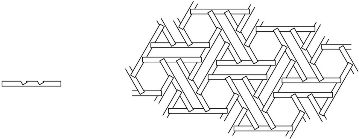
**Figure 7: Hexagonal lattice produced from an asymmetrical part.**
