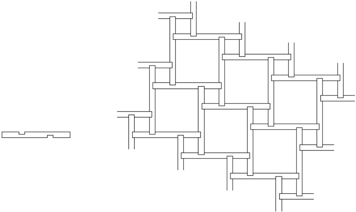
**Figure 5: Linear counterchange lattice and its component part.**
