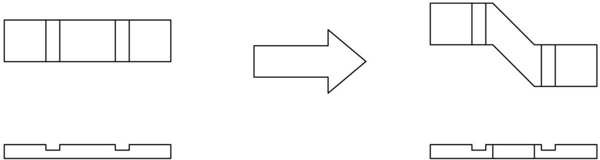
**Figure 8: Mirrored counterchange lattice component stretched upward parallel to the dados.**
