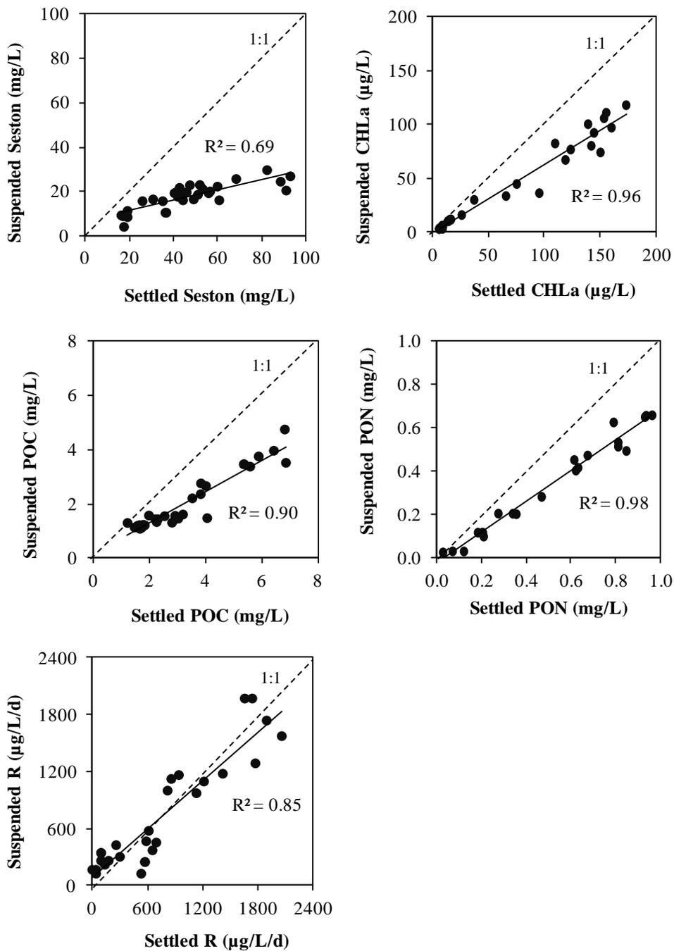
**Figure 7.** Constituent concentrations in the upper (suspended) and lower (settled) halves of the settling tubes after 240 minutes. Seston, CHLa, POC, and PON all had measurable differences between the two halves as is evidenced with data points falling below the 1:1 line. The exception was respiration - differences between the upper and lower halves were indistinguishable.
