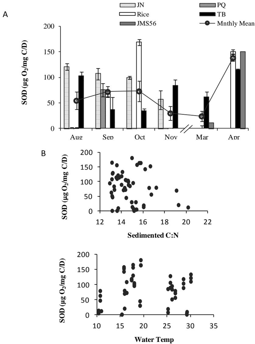
**Figure 6.** A) Sediment oxygen demand (SOD) by site and month. (Error bars are standard error.) B) The relationship between SOD and water temperature and SOD and sediment C/N.
