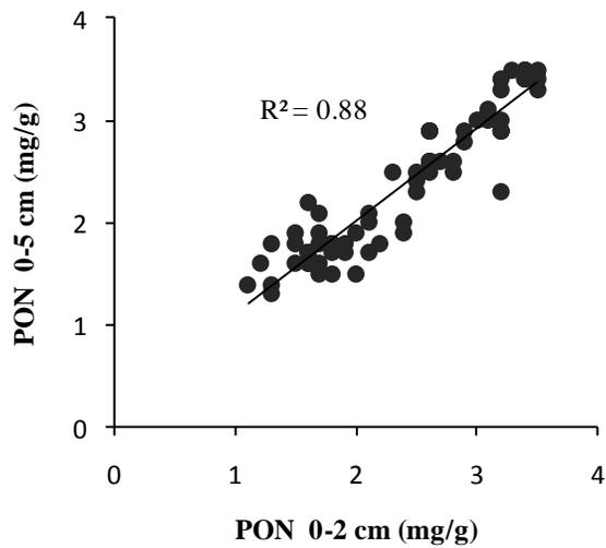
**Appendix Figure 2.** Relationship between 0-2 and 0-5 cm cores for POC and PON. Proportional differences between 0-2 and 0-5 cm cores are minimal. Therefore all results reported in this study are based on the 0-2 cm cores. Linear regressions are significant ( $P < .05$ ).
