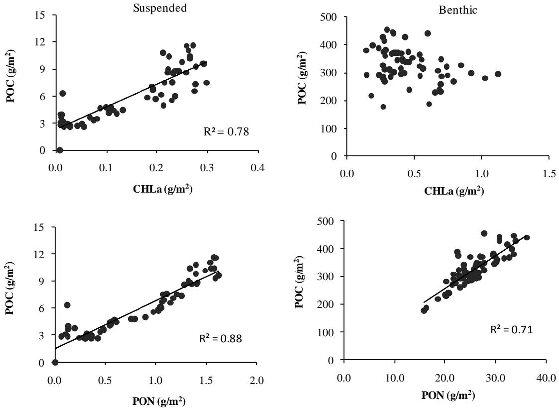
**Figure 4.** A) The positive correlations between suspended POC and CHLa suggest that phytoplankton is a significant contributor to organic matter in the tidal freshwater James River. B) POC and PON were well correlated for both suspended and benthic sediments. Overall, the larger scales on the x and y axes of the benthic plots indicate increased constituent masses in the benthos relative to suspended masses. Linear regressions are significant ( $P < .05$ ).
