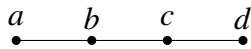
Figure 1.18: For this graph, \{bc\} is a matching but it is not a maximum matching, whereas, \{ab, cd\} is a maximum matching.
