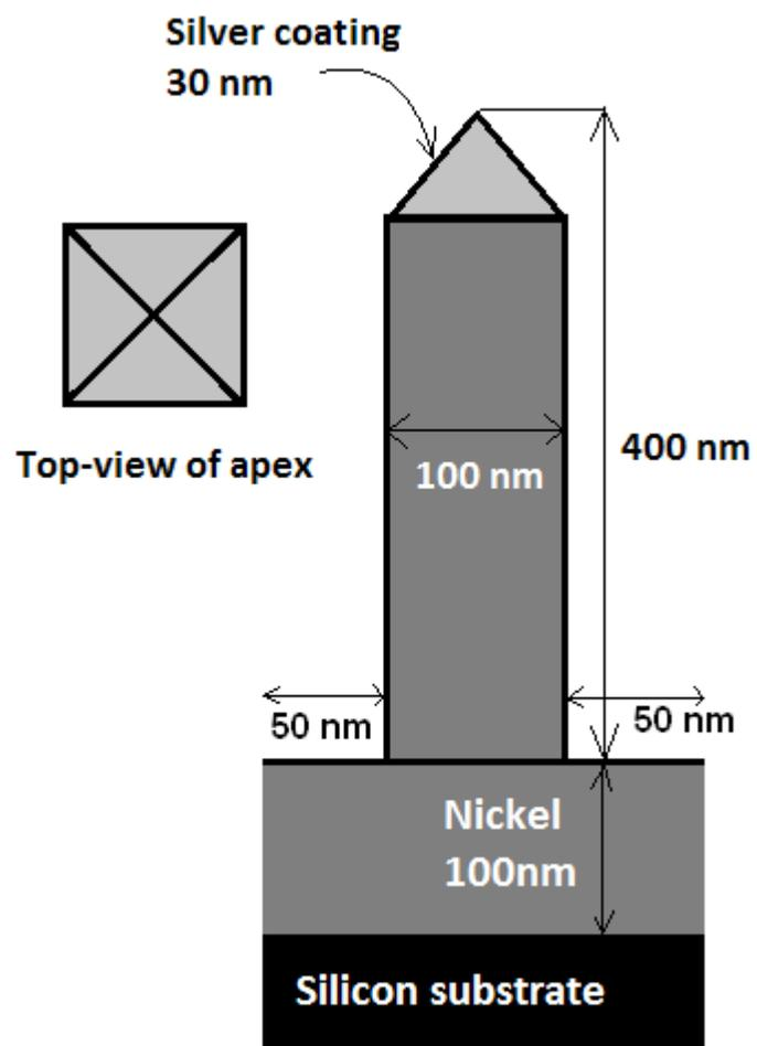
**Figure 4.** Diagram of the simulated nickel nanorod with silver tip.
