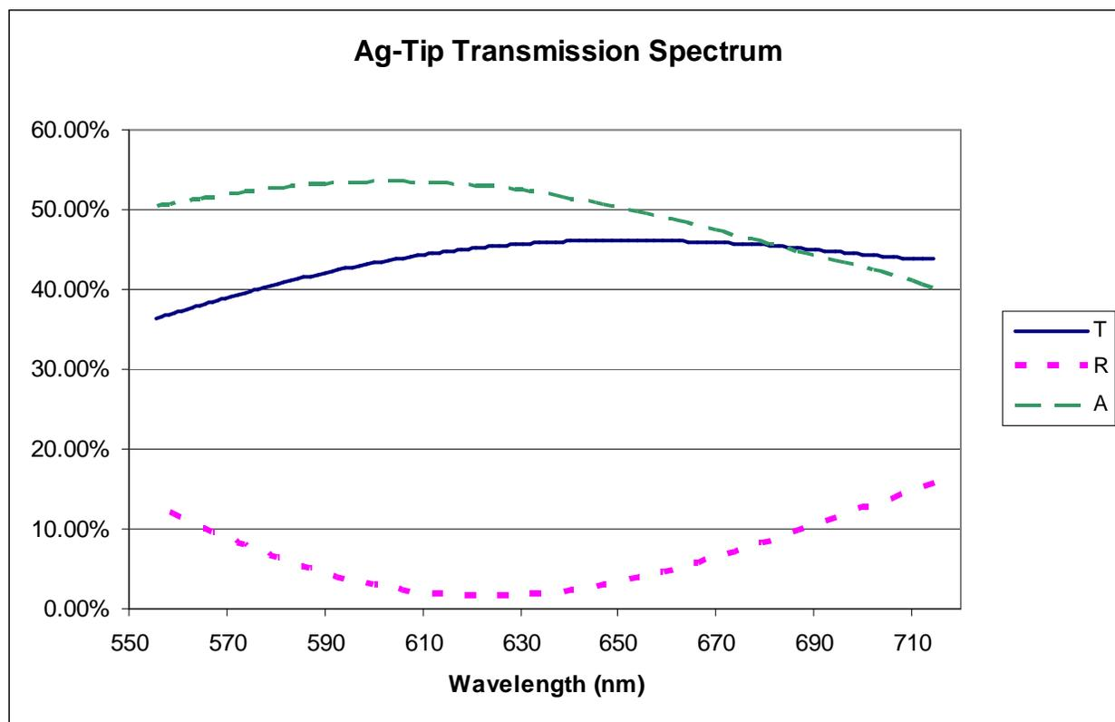
**Figure 5:** A typical absorption-reflection-transmission spectrum for the nickel nanotip with silver thin film. The main features include a minimum for the reflectance, as well as maximum values for both transmission and absorption.
