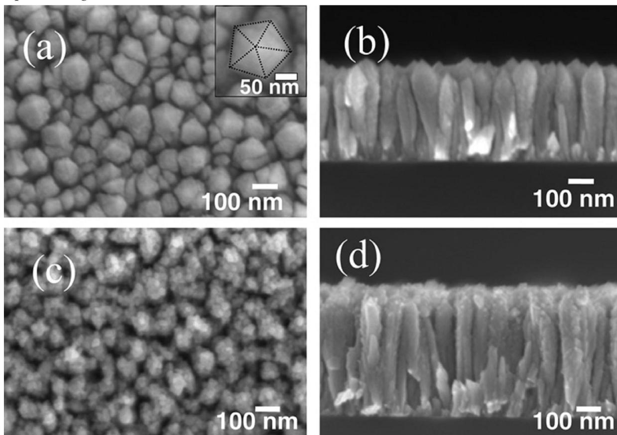
**Figure 1:** Fabricated Ni nanotips top view (a), and side view (b) via scanning electron microscopy (SEM). Also, said Ni nanotips with a 30nm silver film deposited on the surface, top view (c) and side view (d).[Ref. 16]
