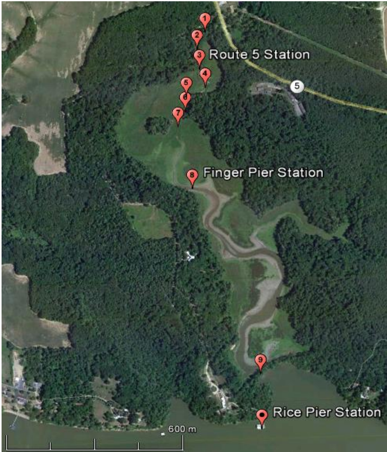
Figure 1: Aerial photo of Kimages Creek showing the sampling locations for the longitudinal survey (sites 1-9) and the current locations of continuous monitoring stations (sites 3 and 8). Note: Seasonal and episodic data comes from the Route 5 sonde when it was located just upstream of site 1).
