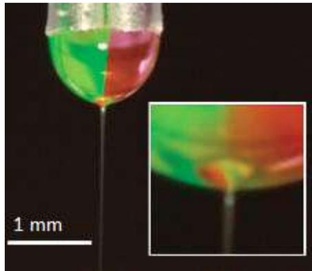
**Figure 7.** Electrospinning of two PEO/distilled water (2% w/v) solutions each mixed with two fluorescent dyes. Left side: isothiocyanate-conjugated dextran (green); Right side: rhodamine-B-conjugated dextran (red). A well-structured side-by-side Taylor cone was observed at the tip of the nozzle, consisting of two aligned fluid phases [37].
