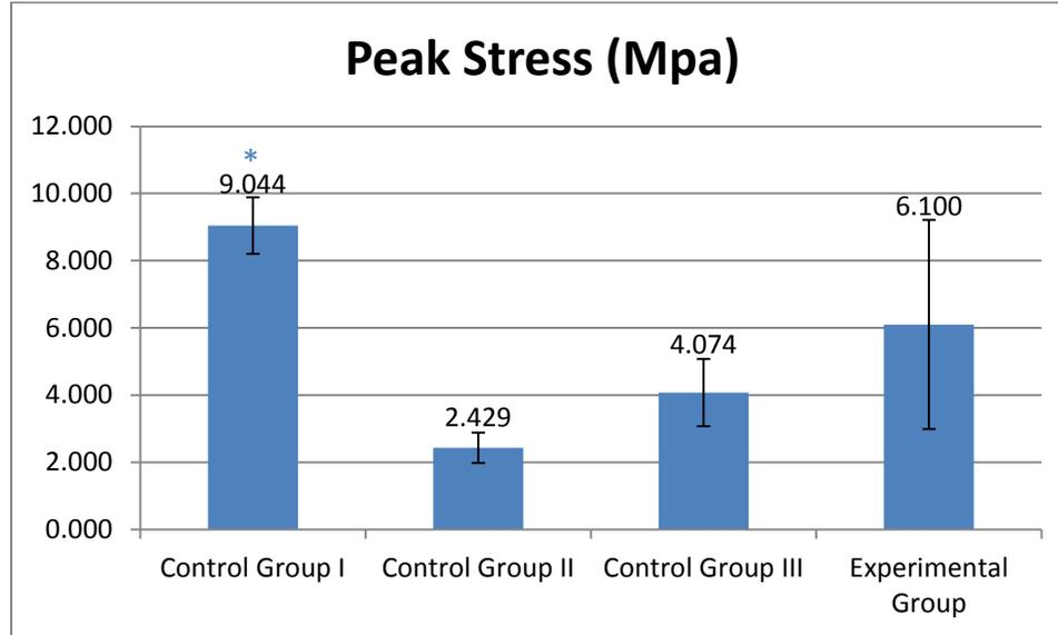
**Figure 12.** Mean peak stress of each group with standard deviations as error bar. (\*) denotes statistical difference ( $p < 0.05$ ) from the other three groups. CII and EX are statistically different ( $p < 0.5$ ) from each other.
