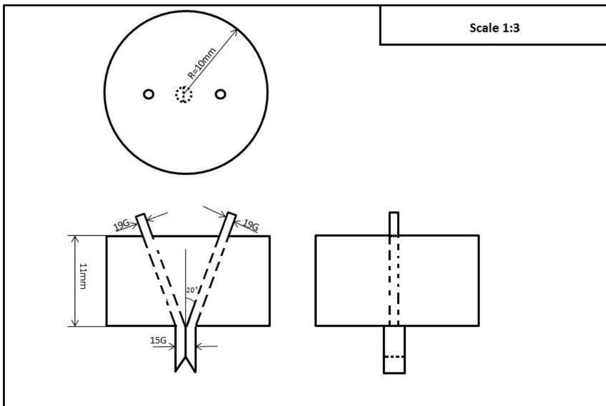
**Figure 20.** An ideal side-by-side bicomponent electrospinning spinneret design.
