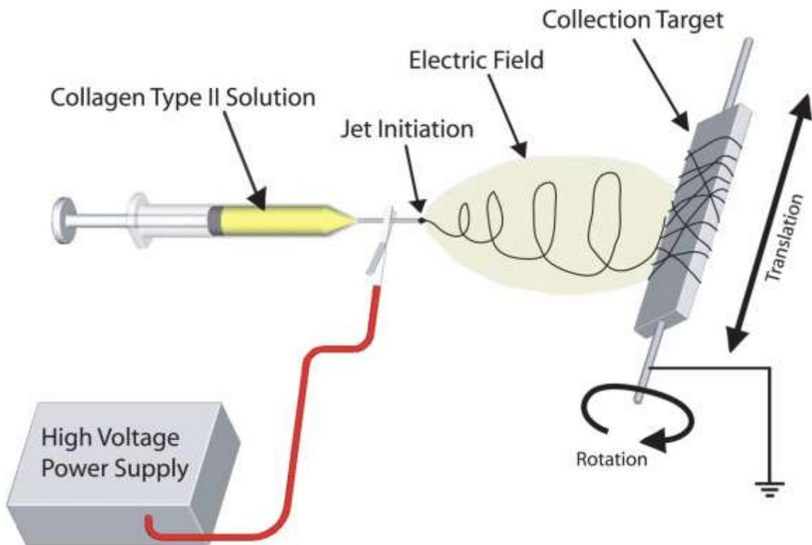
**Figure 2.** Schematic of the electrospinning process to illustrate the basic phenomena and process components [11].
