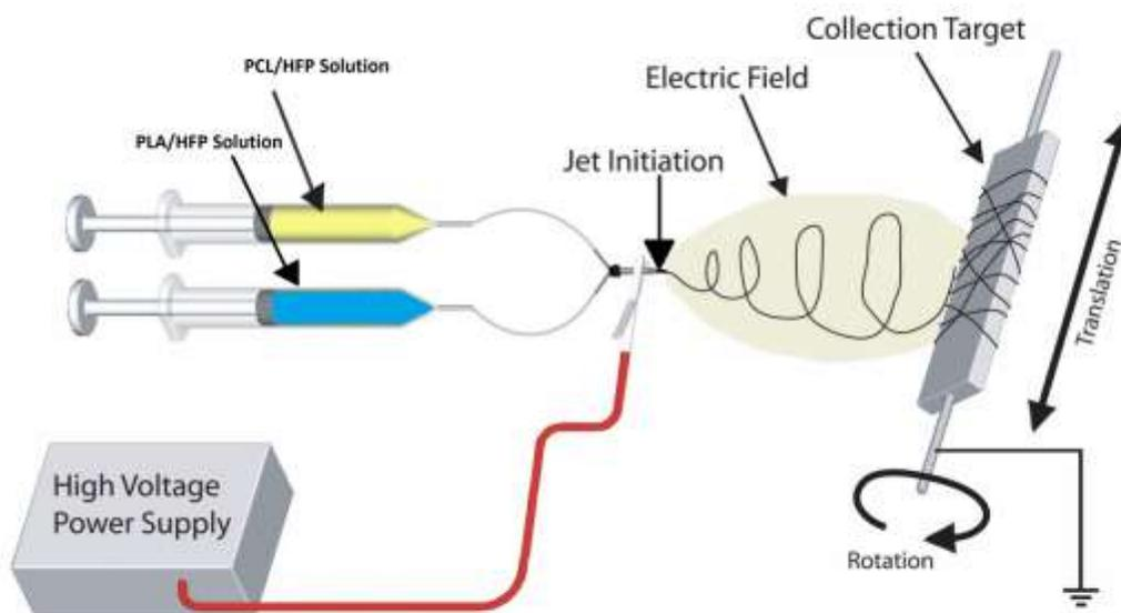
**Figure 4.** Electrospinning setup for side-by-side bicomponent material.
