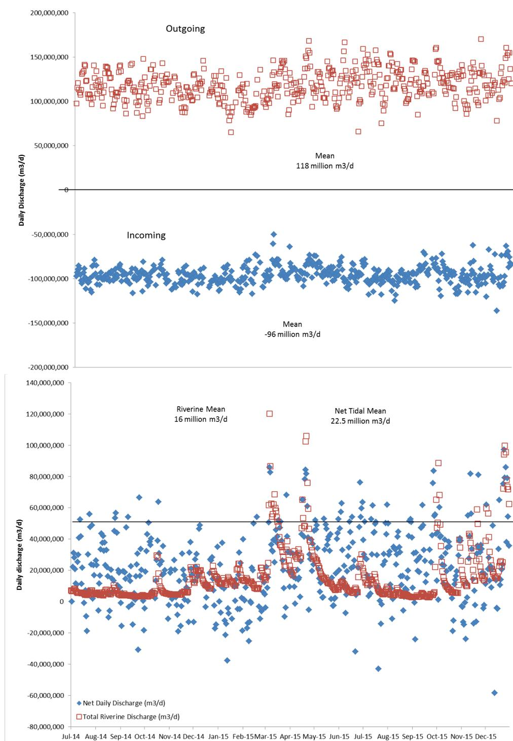
Figure 5. Upper panel: Daily total discharge ( $\text{m}^3/\text{d}$ ) of incoming and outgoing tides at Point Weyanoke, VA. Lower panel: Net daily discharge from Point Weyanoke, VA compared to total daily riverine discharge. Riverine discharge calculated by summing daily discharge measurements from Appomattox River at Matoaca (#02041650), James River near Richmond (#02037500), and James River and Kanawha Canal near Richmond (#02037000).
