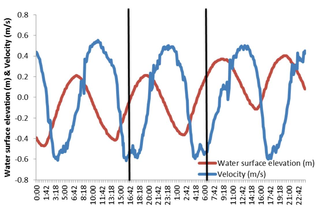
Figure 4. Water velocity (m/s) and surface elevation (m) of the James River at Point Weyanoke during February 25-26, 2015. Black lines denote the beginning and end of a tidal cycle during which an ISCO sampler was deployed to collect samples at 1-h intervals.
