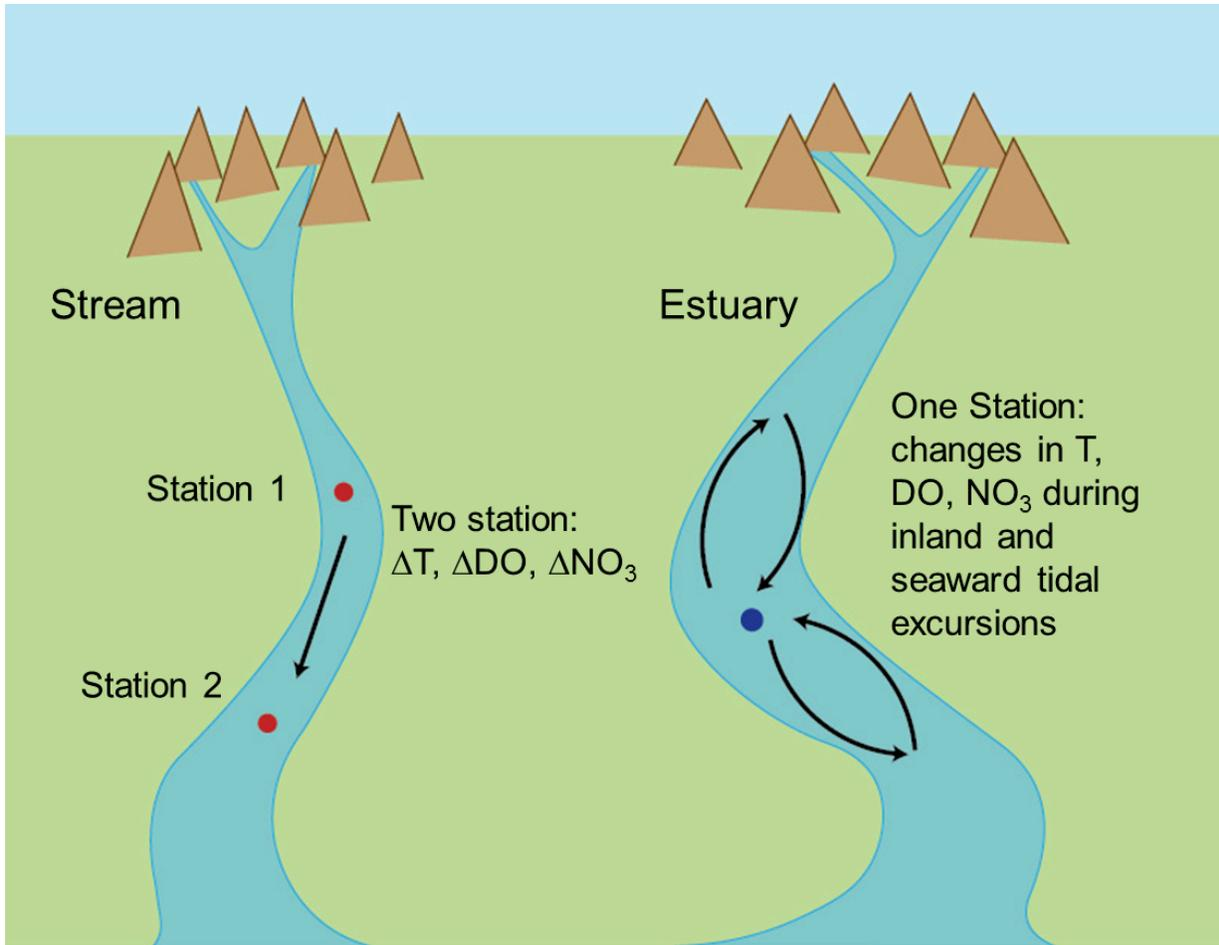
Figure 3. Comparison of how metabolism can be measured in flowing waters. Left: Uni-directional flow allows one to measure changes in temperature (T), dissolved oxygen (DO), and nitrate ( $NO_3$ ) that occur between a station upstream and downstream. Right: Bi-directional due to the tides allows one to measure changes that occur between tides in both directions from one site (excursion analysis).
