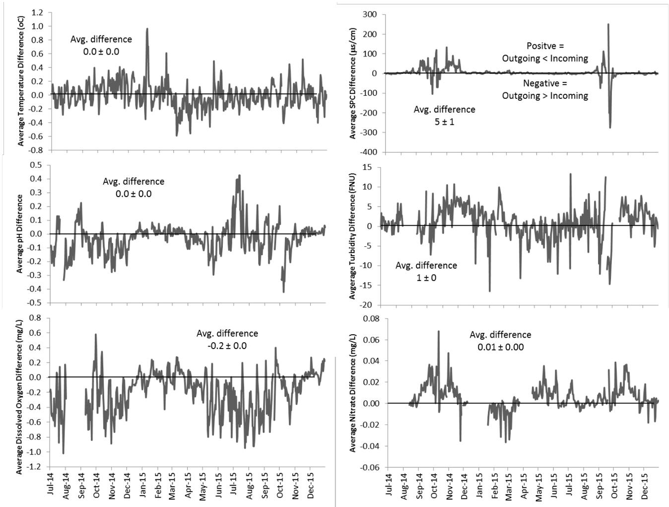
Figure 7. Daily average differences between incoming and outgoing tides for water temperature, specific conductance, pH, turbidity, dissolved oxygen, and nitrate from July 2014 to December 2015 at Point Weyanoke, VA.
