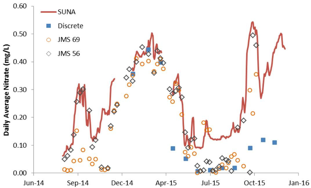
Figure 10. Comparison of nitrate concentrations between the continuous SUNA data (Point Weyanoke), monthly discrete samples (Point Weyanoke), and weekly sampling at James River mile 56, and 69.
