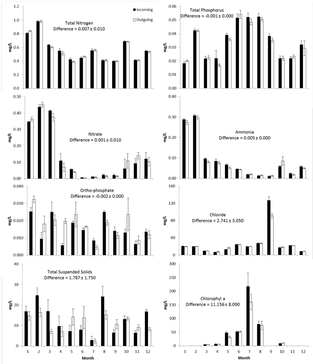
Figure 8. Average total nitrogen, total phosphorus, nitrate, ammonia, ortho-phosphate, chloride, total suspended solids, chlorophyll a, particulate organic carbon, and particulate organic nitrogen from monthly discrete samples for incoming and outgoing tides at Point Weyanoke, VA. Chlorophyll a only measured March – August and October 2015.
