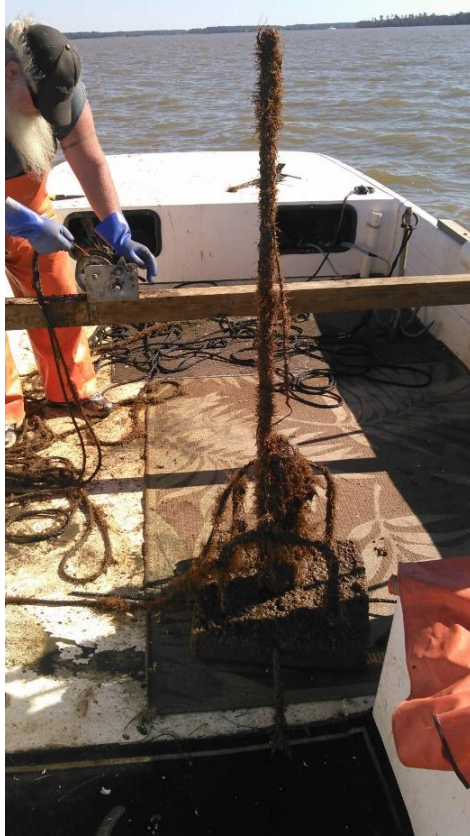
Figure 1. Retrieved receiver mount from the dredge site array. A concrete base with steel rebar keeps the receiver at the bottom of the river oriented vertically. The long vertical piece of rebar has a synchronization tag at the top to allow the array to detect drifts of receivers for accuracy.
